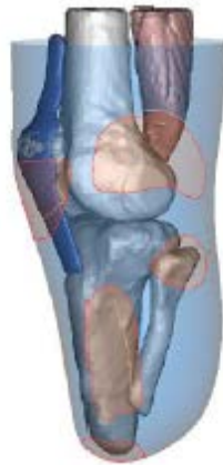
Figure 5: Highlighted areas to be modified for an effective socket design, with patient anatomy present to inform decisions
