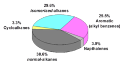
Figure 2.15. The molecular class distribution of the Jet A POSF 4658 fuel from gas chromatographic/mass spectrographic detailed analyses reported in [64]. The summary figure
