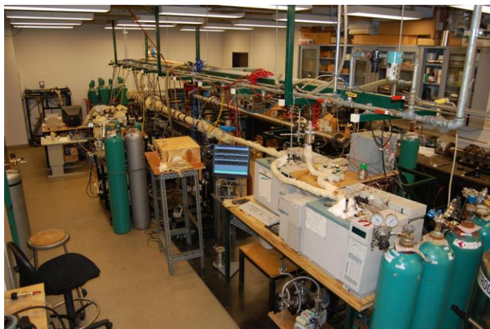
Figure 6.1 The heated high-pressure single-pulse shock tube; performance range 15-1000 atm, 900 to 2500K, 0.5 to 3 msec.
