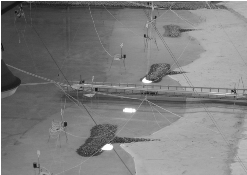
Fig. 4. Physical model oblique view showing profile measurement location and bridge.
