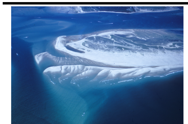
Figure 9. Oblique aerial photo of Monomoy Island (MA) spit at low tide (circa 1970) showing trailing, ebb-tidal delta shoals welding to the updrift beach. This process is considered analogous to spit growth at western Fire Island between 1825 and 1940, prior to jetty construction. (Source photo: Courtesy of Miles O. Hayes, Research Planning, Inc.)
