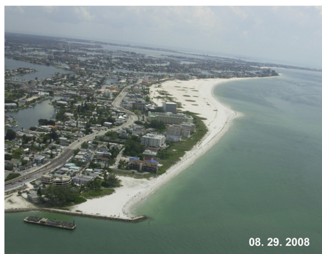
Fig. 6. The attachment point of the John's Pass ebb-tidal delta, where bypassed sand reaches the downdrift shoreline. Note the wide beach at the attachment point, the narrow Sunshine Beach north of the attachment point, and the wide beach south of the attachment point. The photo was taken in 2008 looking south.
