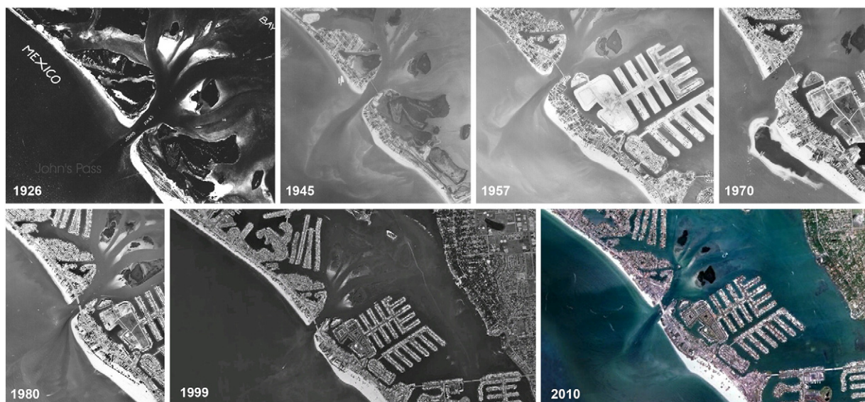
Fig. 4. Time-series aerial photos of John's Pass from 1926 to 2010. Note the relatively stable flood tidal delta, the shoreline variation near the inlet, and the nearshore berm nourishment shown on the 1970 photo.
