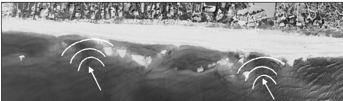
Figure 1. Gaps in bars (marked with arrows) allow higher waves to approach closer to shore, which proceed by diffraction through the gaps
