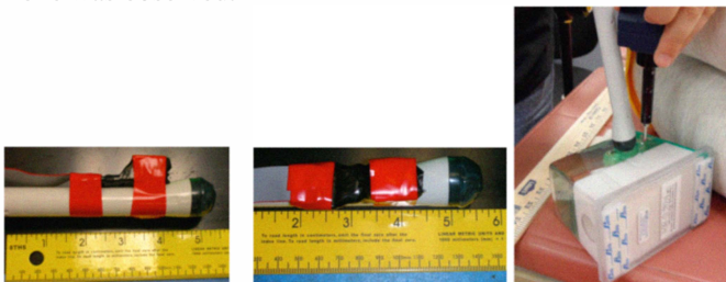
Figure 15. Interference tests performed with the commercial in vitro 3D elastography probe, model Ultrasonix 4DEC9-5/10. Left and center: One of the many tests, here with the small PET probe variant based on a 16ch Hamamatsu MPPC array taped to the US probe. At right is the probe positioning during the test of the interference on US operation from the active Microscribe probe (during position data collection by the position probe). Both probes are placed on top of the commercial elastography prostate phantom [13]. No interference was detected.
