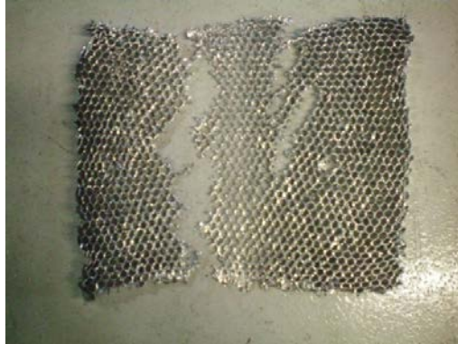
Figure D-1. Material A1 Post Impact.
