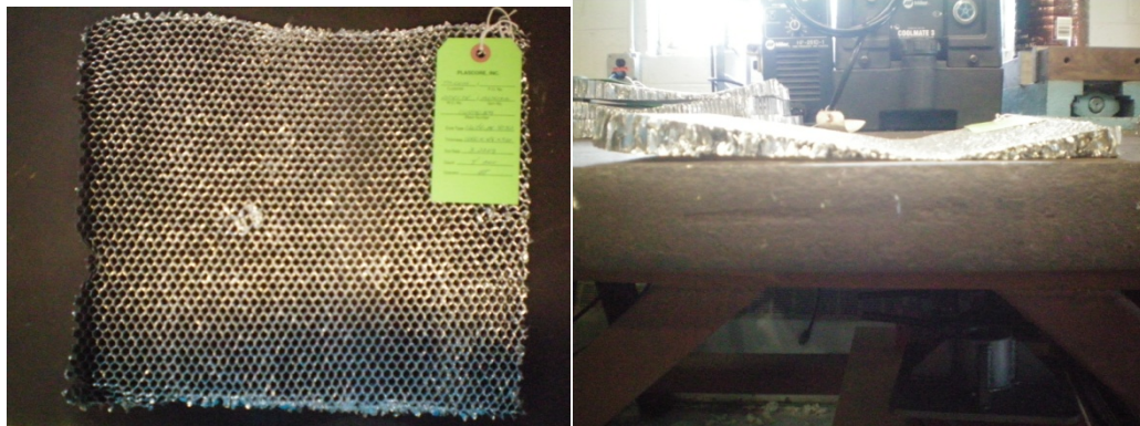
Figure D-2. Material A2 Post Impact.
