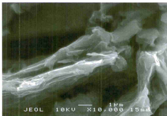
Figure 4: SEM image of the graphene oxide taken at 10KV.
