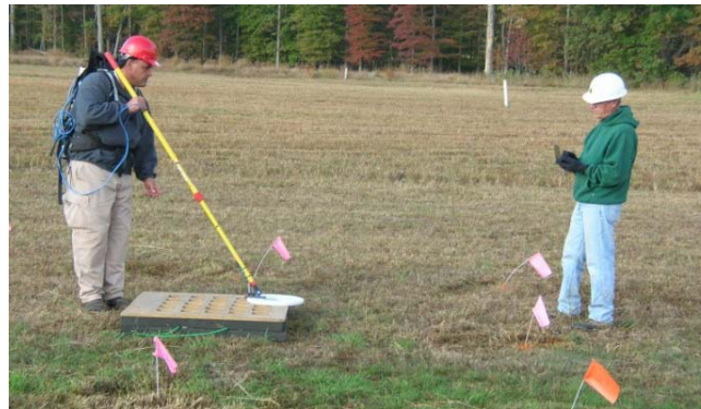
Figure 8. The NRL TEMTADS hand-held sensor.
