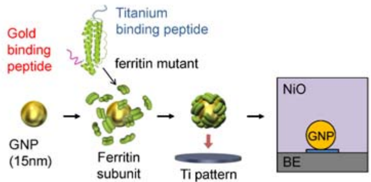
Fig. 2.1 Schematic image of bifunctional protein-based encapsulation/delivery system for nanoscale positioning of a GNP on bottom electrode (BE).
