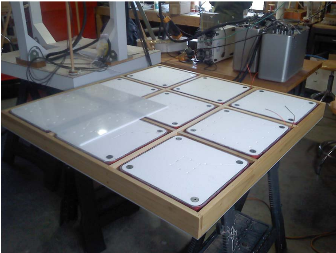
Figure 3.2: Pedemis Tx array. Tx loops are the same size and template as the TEMTADS coils. 35cm loop size with 40cm between centers. See Sec. 3.2.a for more information about the Pedemis transmitter array.
