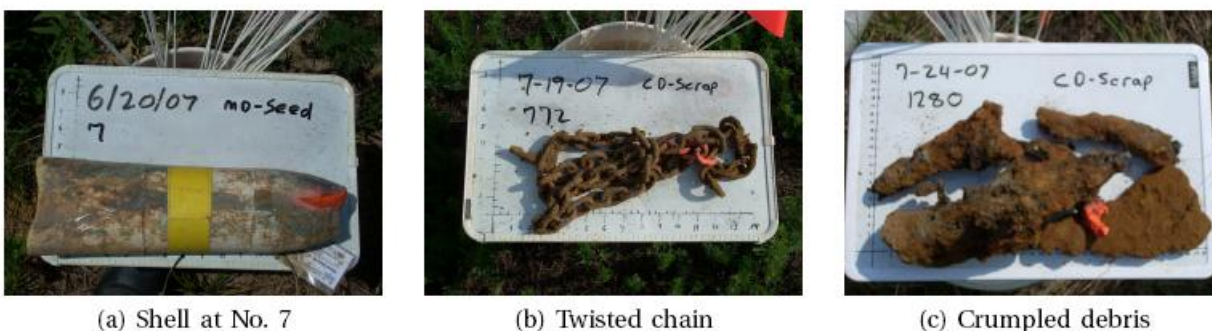
Figure 36: a) Unexploded shell from Cell No. 7 and (b,c) the two false alarms obtained by the SVM classifier using k and Q(t_{15})/Q(t_1) as discriminators.
