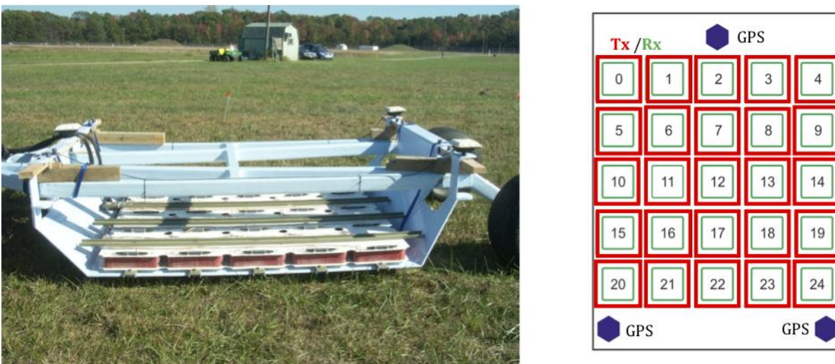
Figure 12: Photo of the TEMTADS in deployment at Blossom Point Test Site (left) and a schematic diagram of its Tx/Rx sensors (right).
