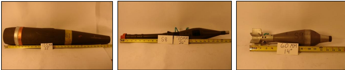
Figure 5. Inert UXO simulators of a 155 mm projectile (left), 70 mm rocket (middle), and 60 mm mortar (right) used as targets to mimic real munitions items for LLSS calibration and validation elements.
