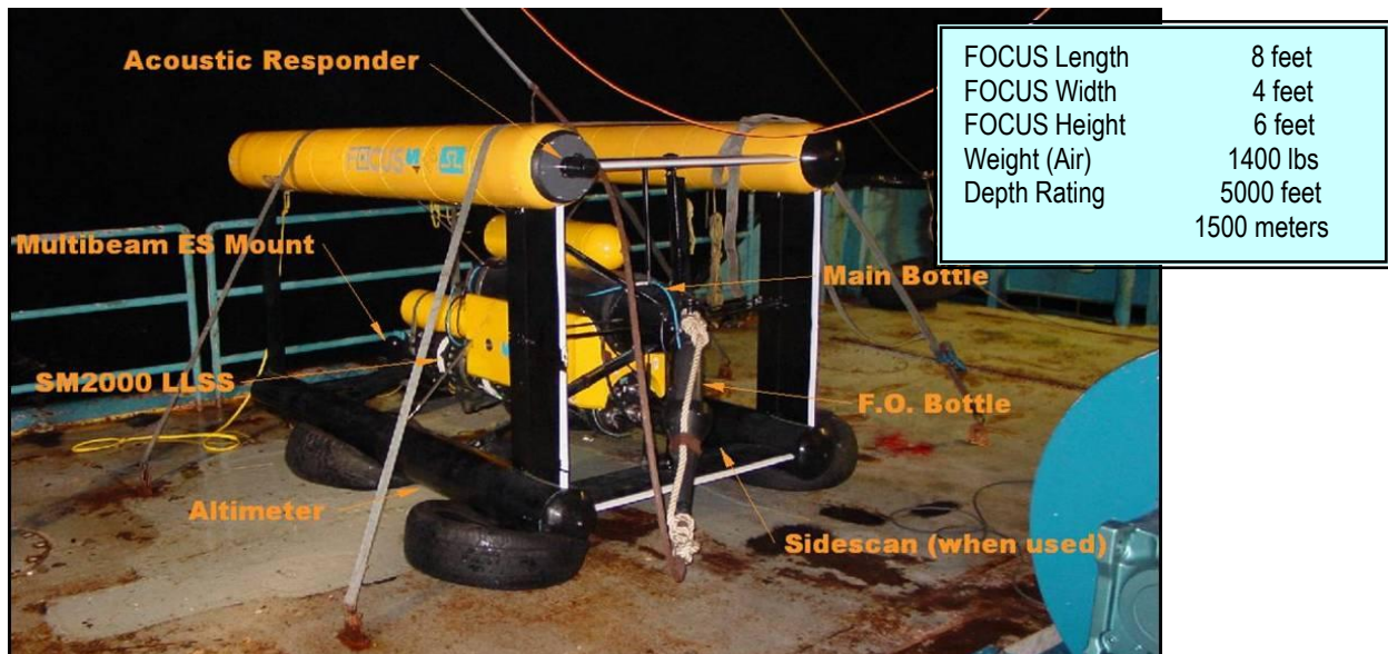
Figure 2. Photo of the FOCUS 1500 system prior to deployment for an offshore survey with major components identified, as well as dimensions and depth rating for the tow body.
