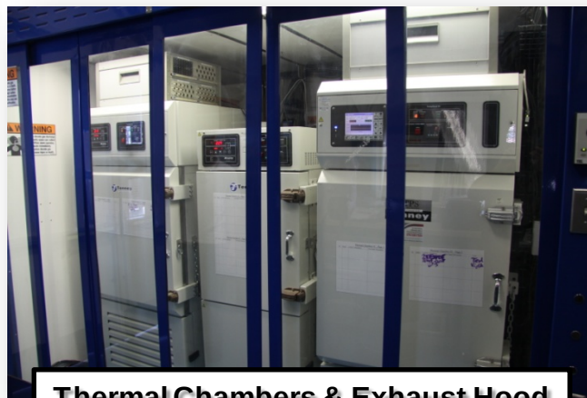
Thermal Chambers & Exhaust Hood
