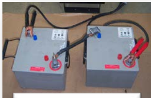
12V Lead-Acid 6T Batteries 80kg total
