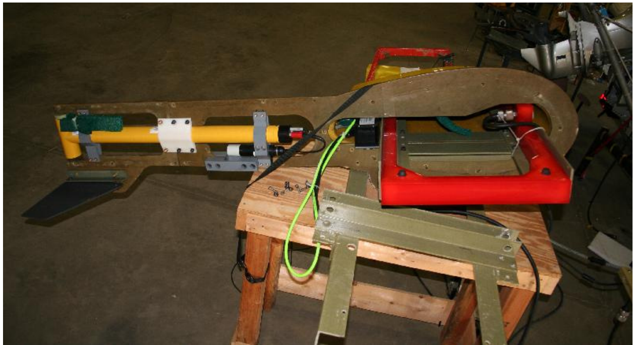
Figure 4: Mag/EM61 towfish internal components
