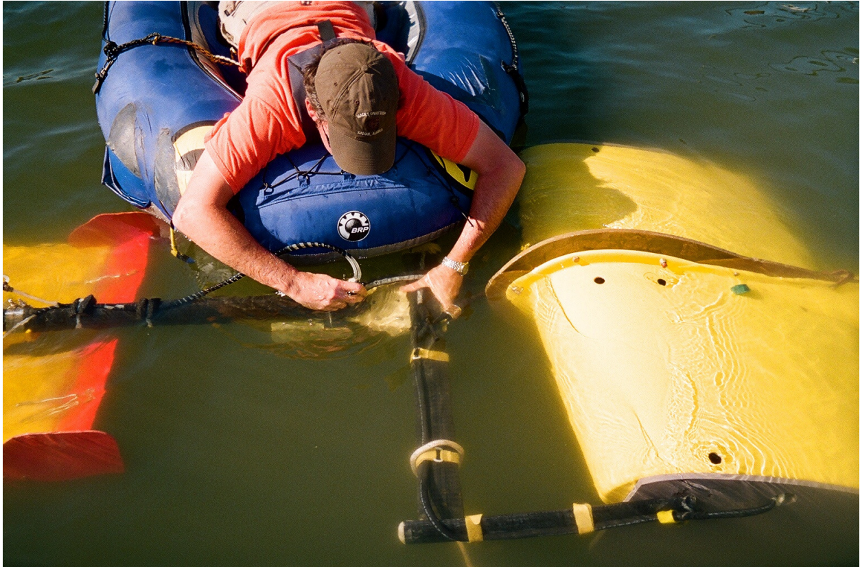
Figure 5: Towfish, bridle, and boom
