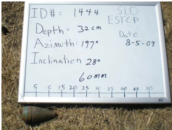
Figure 7-5. Photograph of target 1444 which is a 60mm body that was classified as high confidence clutter.
