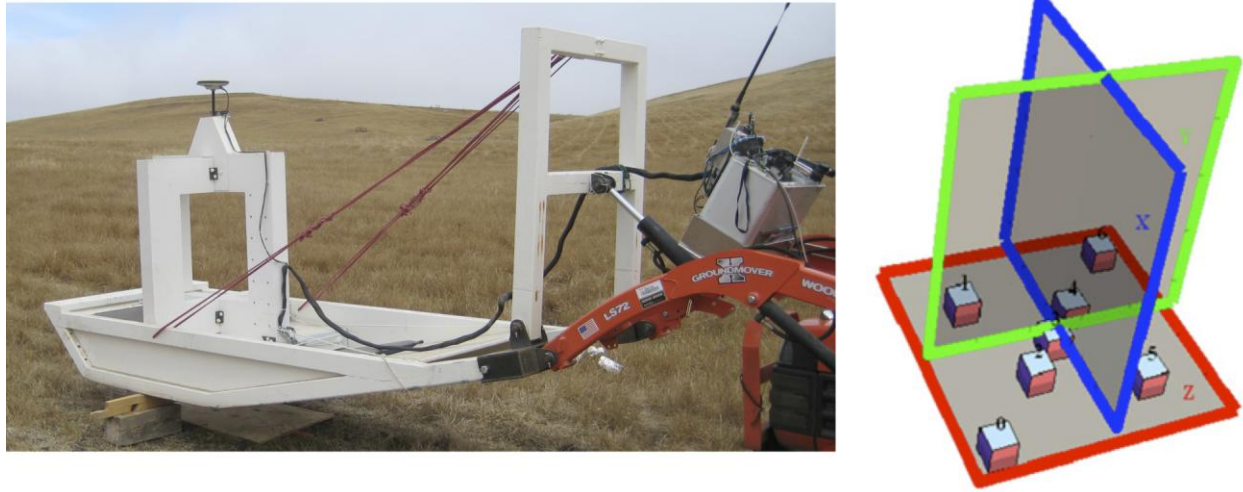
Figure 1: The MetalMapper during SLO site deployment (left) and its schematic diagram (right).
