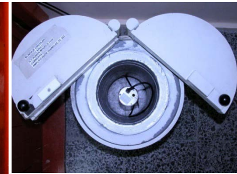
View of Test Chambers (top), Gieger Mueller and NaI Detectors with ^{54}\text{Mn} , ^{32}\text{Si} , ^{36}\text{Cl} , ^{90}\text{Sr} , and empty NaI detector
