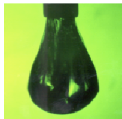
a) \text{MnO}_2 film formation on a TCE droplet in water.
