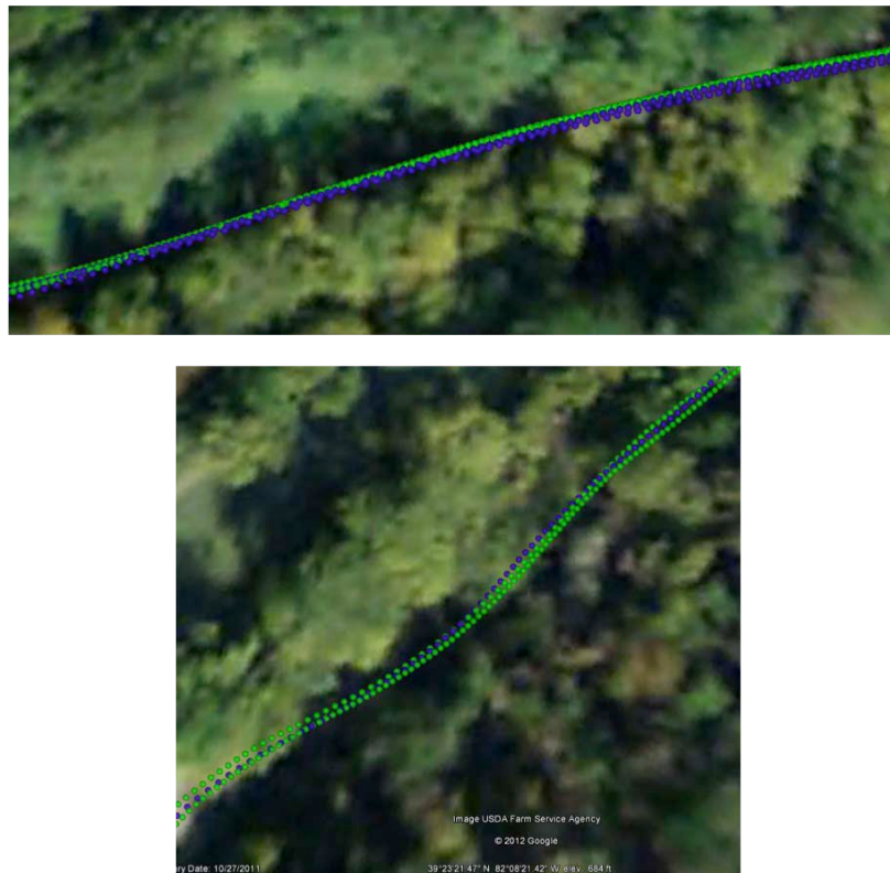
Figure 4.13 Trajectory reconstruction consistency for multiple tests: Google Earth representation of deep integration position estimation results; green and blue dots correspond to two independent test trajectories driven along the same path; zooming on select test segments
