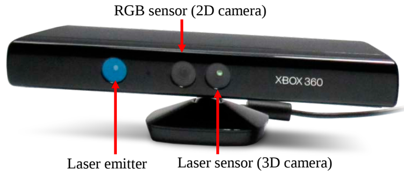
Figure 6.1 Kinect XBOX 3600 sensor, including 2D and 3D imaging sensors
