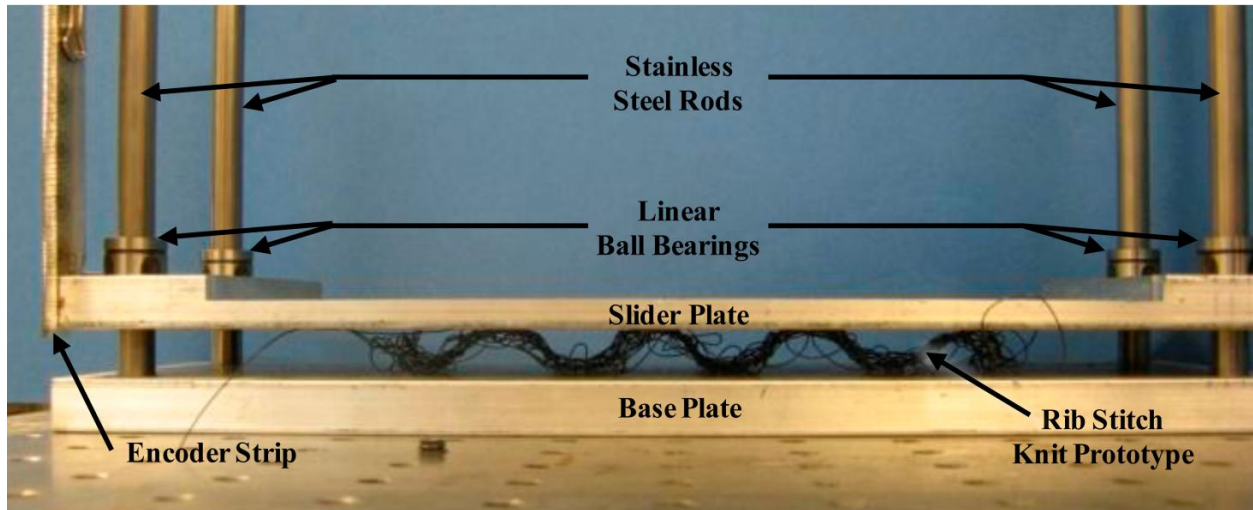
Figure 32. Experimental Setup for Testing of Rib Stitch Knitted Prototypes. The rib stitch prototype expands from the Martensite Compressed State to the Austenite Expanded State to lift the slider plate and any additional applied loads.
