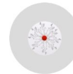
Nano-Al Encapsulated with Ammonium Perchlorate
