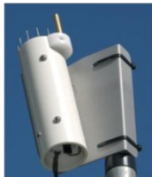
Boltwood Cloud Sensor
