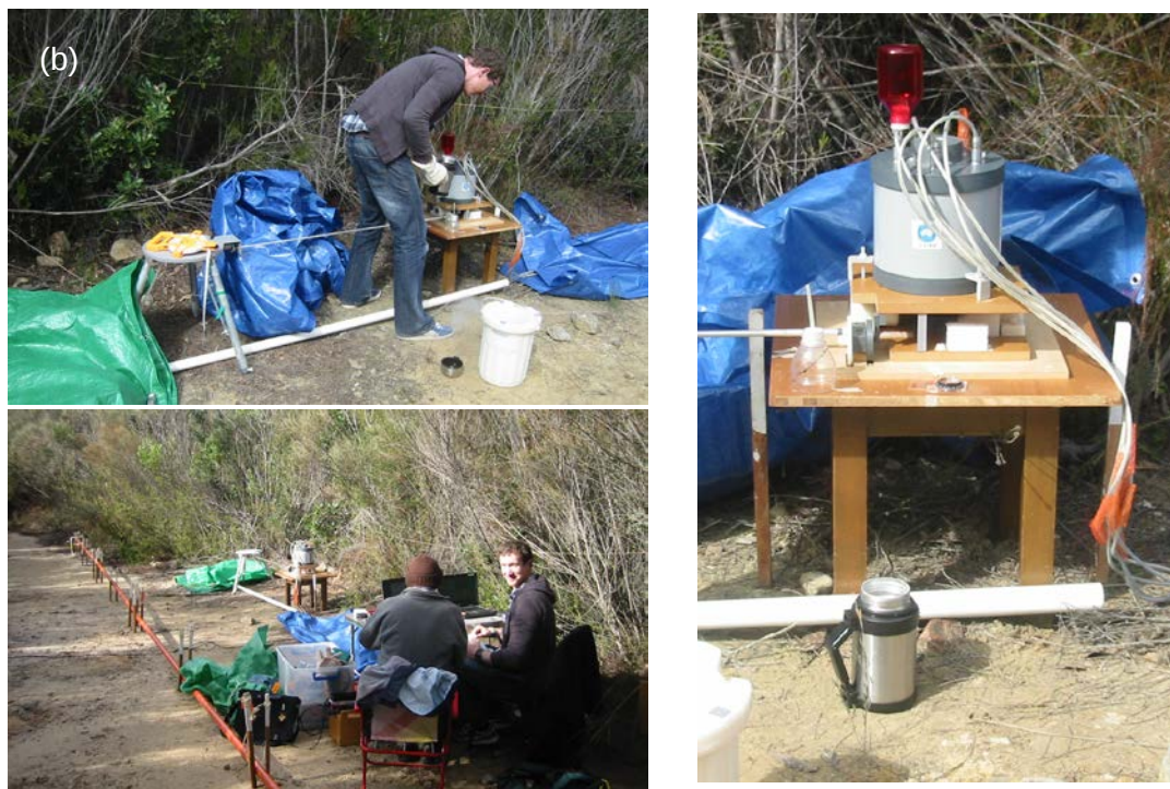
Figure 63. (a) A Google map image showing the route take to the West Head trial site from the Lindfield labs with the inset showing the exact location of the system. (b) shows a number of photos from the trial. Top left: initial cooling of the system using \text{LN}_2 showing the system mounted on the tilt table and drive shaft to a dc motor mounted on a tripod. Right shows a close up of the system.
