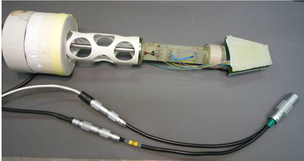
Figure 15. Custom built 2-channel noise measurement probe with a mounted device ready to test, with LEMO connectors .
