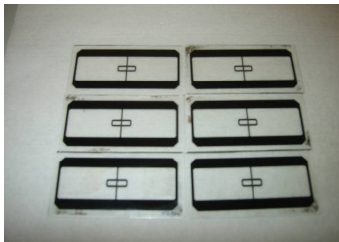
Figure 33. Six design C gradiometric antennas before flip-chipping.
