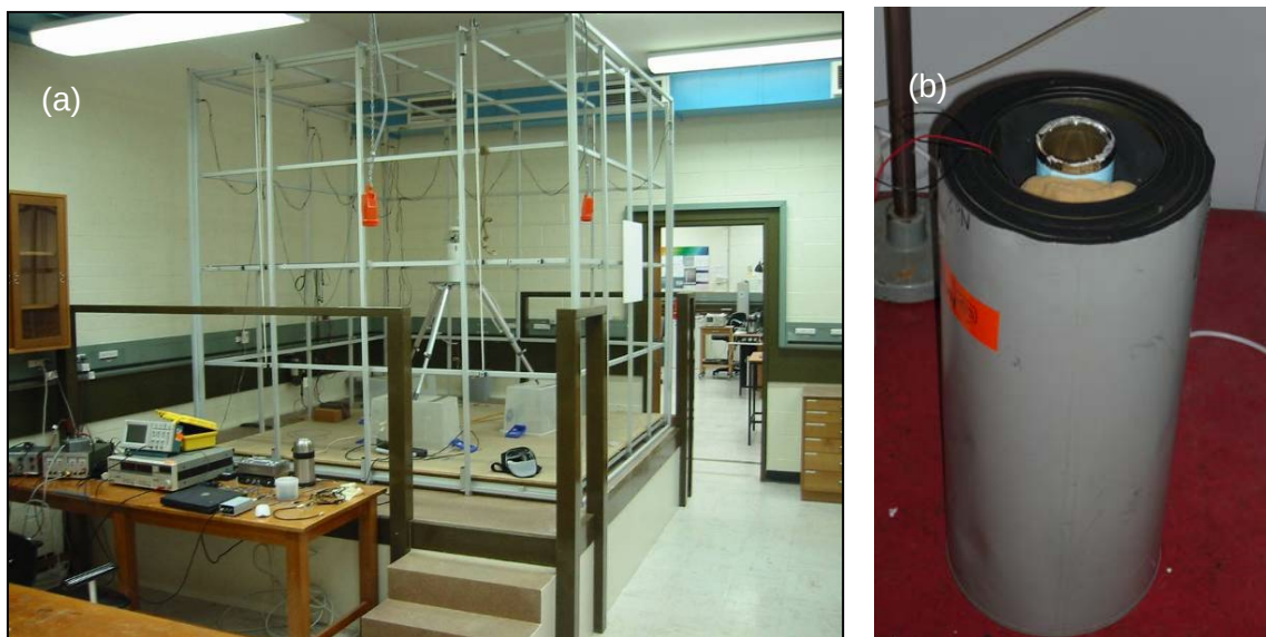
Figure 53. (a) The 2.5 m outer diameter, tri-axial Ruben's coil set in the Lindfield CSIRO laboratory and (b) mu-metal shielding used to measure the intrinsic noise of the devices.
