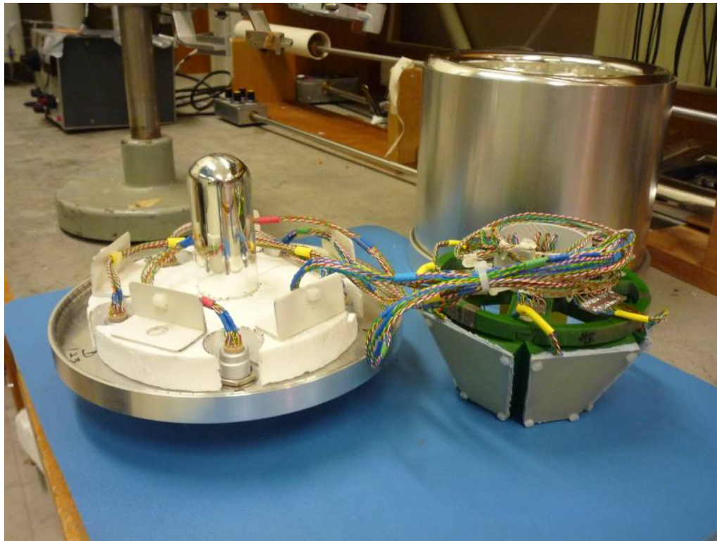
Figure 44. Wiring for the full system, with a total 108 wires (54 twisted pairs).
