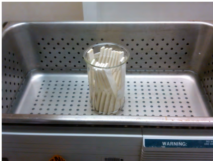
Figure 6.12: DNS specimens during 25 minute ultrasonic acetone bath
