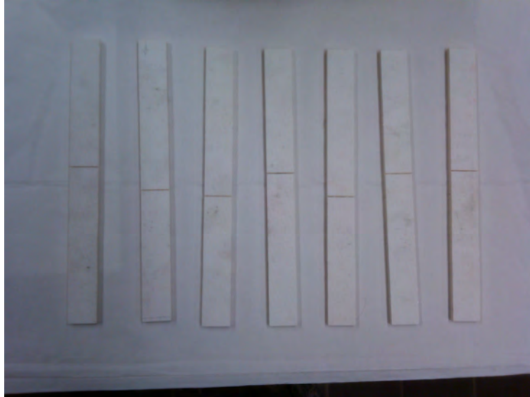
Figure 6.9: DNS specimens before cleaning
