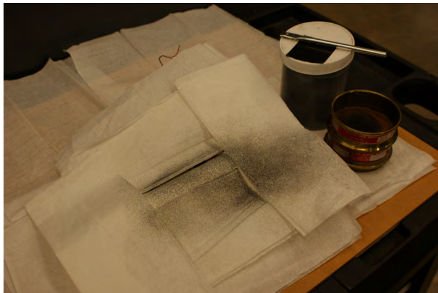
Figure 4.23: Laser printer toner speckling procedure on involute oxide-oxide CMC tube
