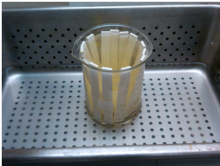
Figure 6.10: DNS specimens during first cleaning
