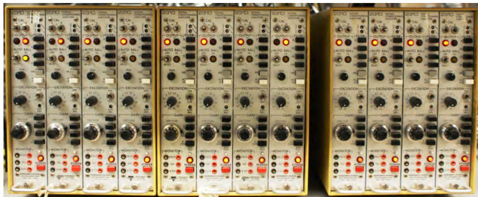
Figure 4.17: Bank of Vishay 2310 rack-mounted strain gage signal conditioning amplifiers
