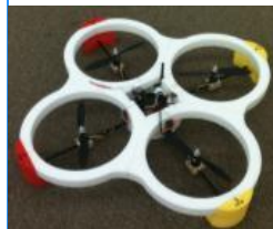
Light-weight in-air module; robotic assembly; variable stiffness material with embedded sensing/actuation
