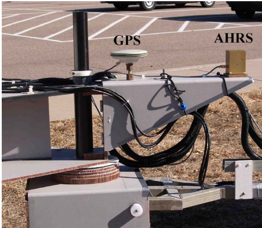
Figure 6. AHRS and GPS antenna on nose of new cart. This photograph shows the forward portion of the ALLTEM cart. The triangular cross-section “nose” extension is the platform for the AHRS, right, and GPS antenna. The AHRS is located far enough away that the electromagnetic interference between AHRS and ALLTEM is acceptably small.
