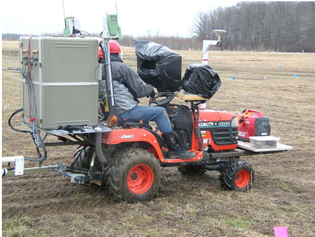
Figure 2. The Kubota tractor used to tow the ALLTEM.
