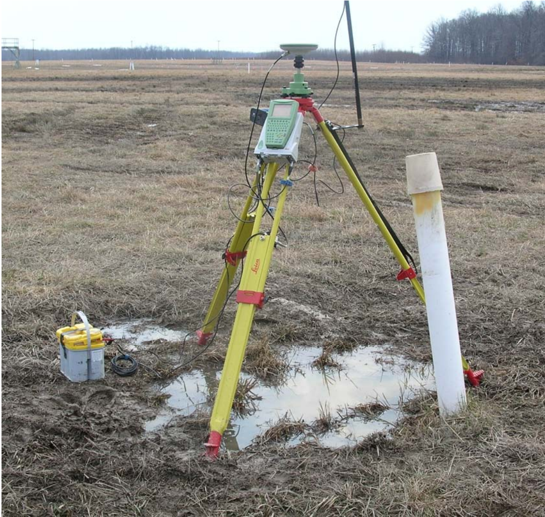
Figure 11. The Leica GPS 1200 base station at APG (marker #477). The monument was typically under a foot of water.
