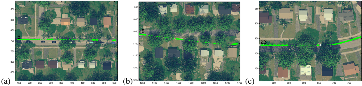
Figure 21: Tracks for three different tracked vehicles. Green dots indicate track updates. Dashed lines connect consecutive updates.
