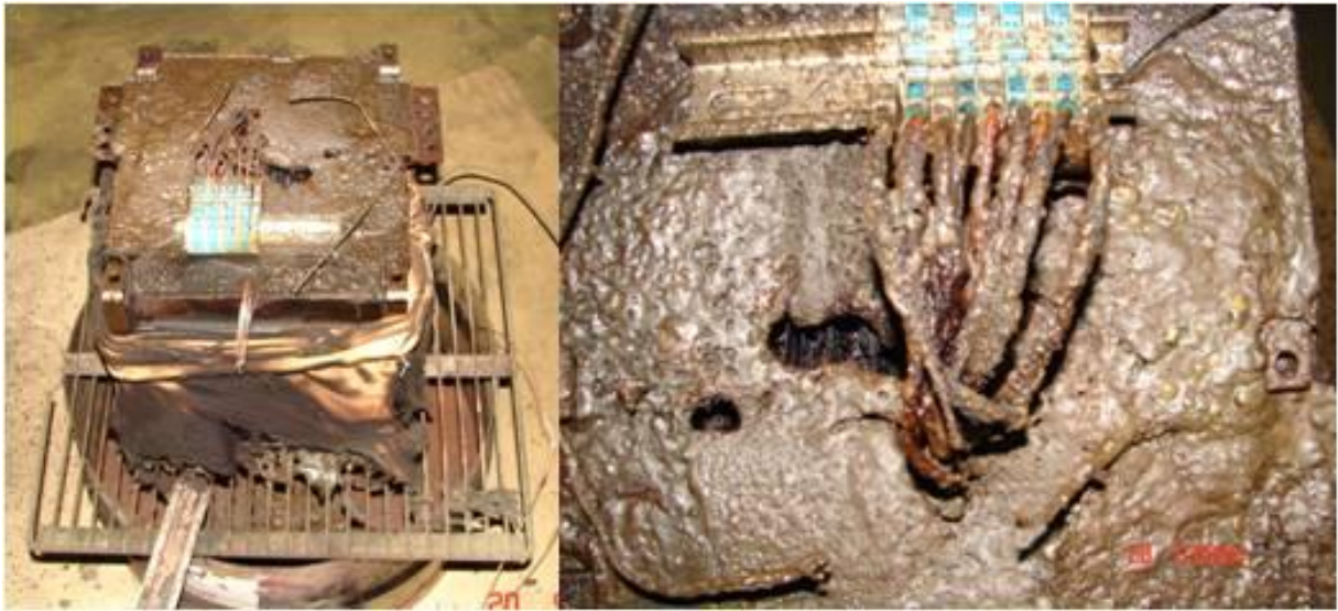
Figure 34: Mark I Module Carbon Dioxide Extinguishing After Test Pictures
