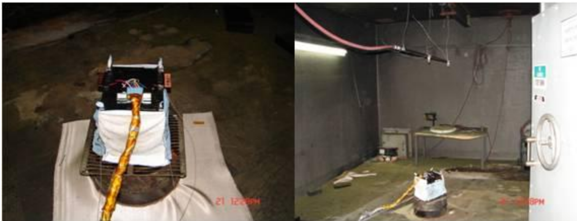
Figure 35: Mark I Module- Water Extinguishing Test Setup
