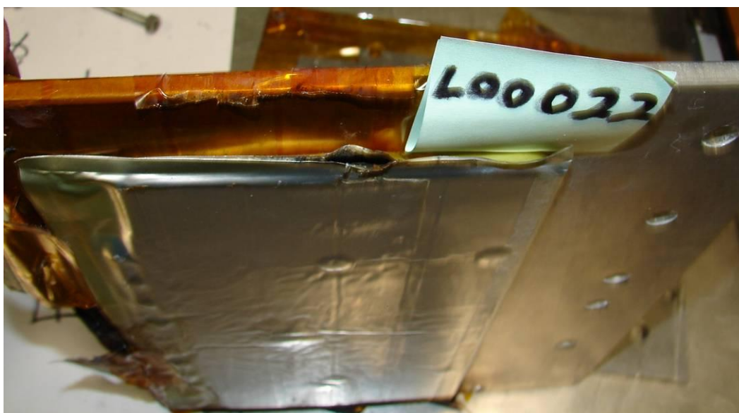
Figure 4: Li-Ion Nano-Titanate Cell Flame Test Cell Damage
