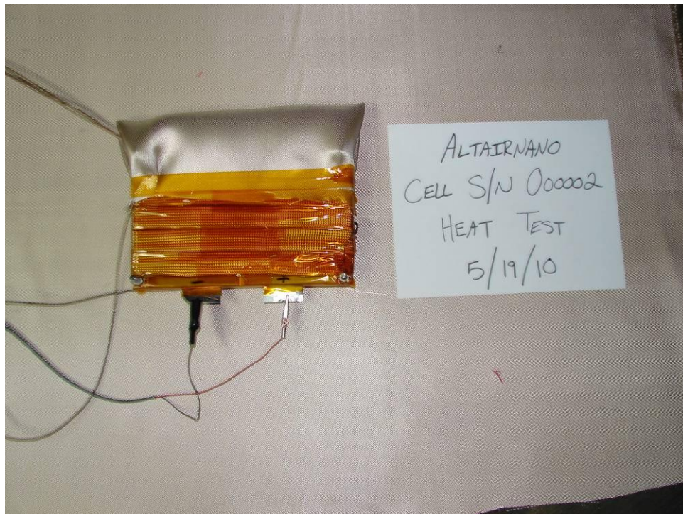
Figure 14 Altairnano Li-Ion Nano-Titanate Heat Tape Test Setup (S/N 000002)
