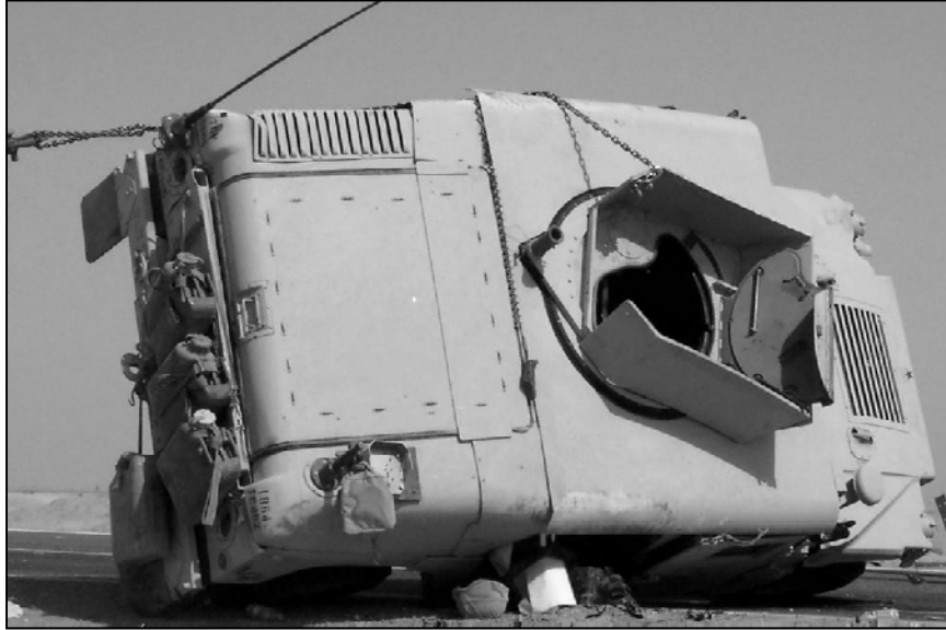
Figure A1. Partial rollover. (U.S. Army photo)
