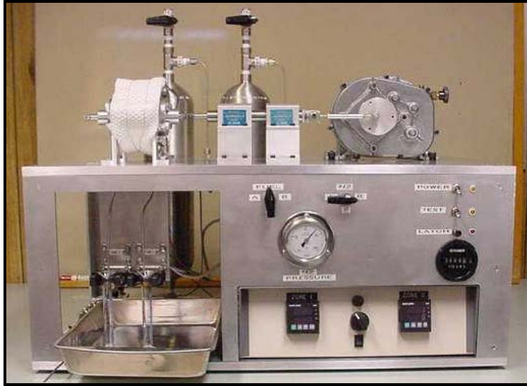
Figure 37. SwRI Dynamic Seal Tester
