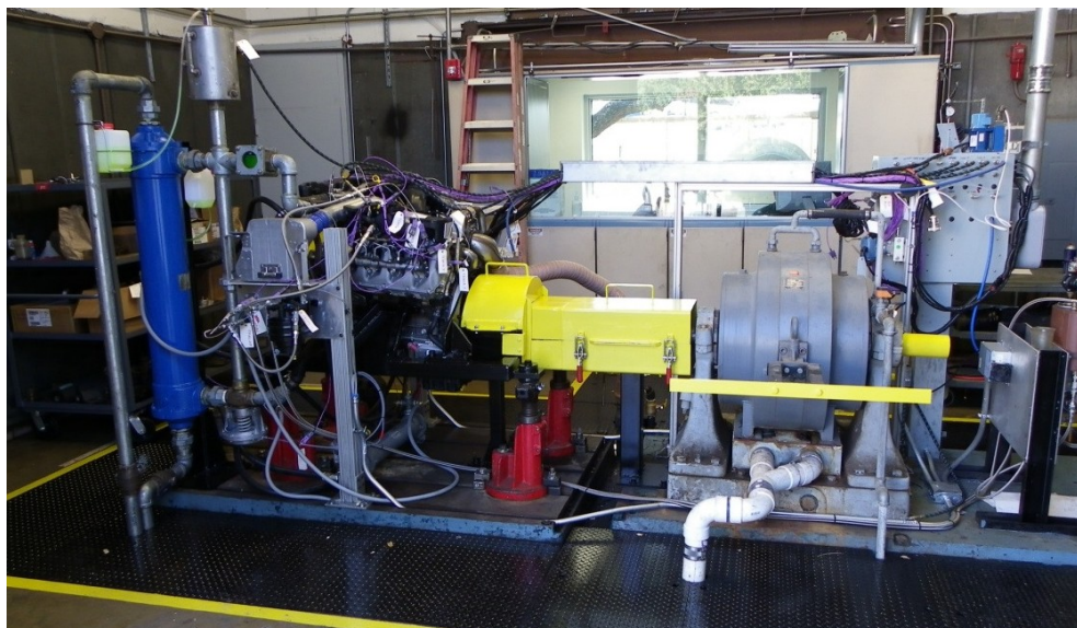
Figure 47. Ford 6.7 L Diesel Engine Test Installation
