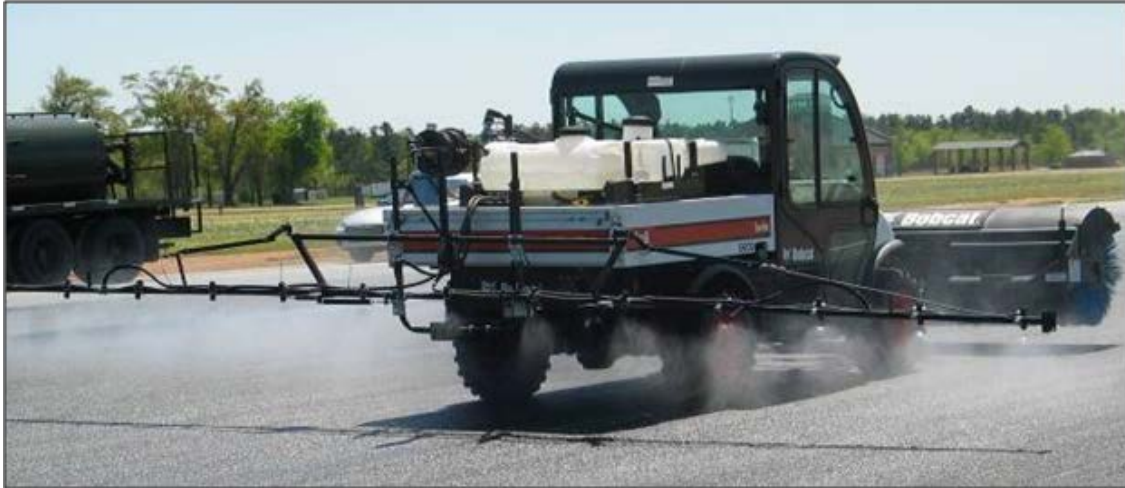
Figure 3. Toolcat ® Applying Detergents with 21-ft Spray Bar
