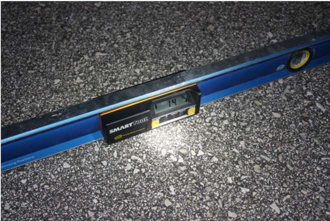
Figure 11. Slope Measurement Reading
