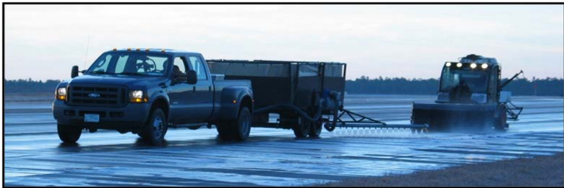
Figure 20. Toolcat ® Applying Detergents to Dampened Test Area
