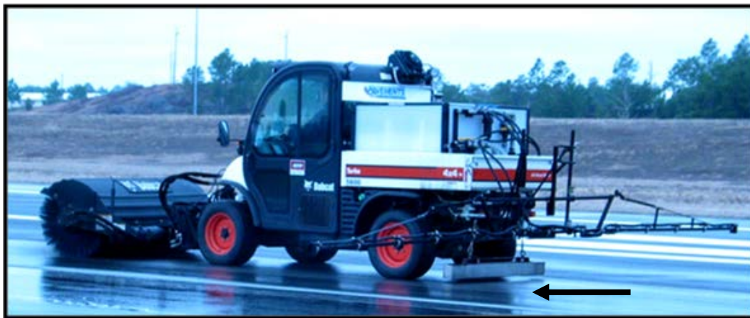
Figure 16. Magnetic Bar Orientation on Toolcat ®
