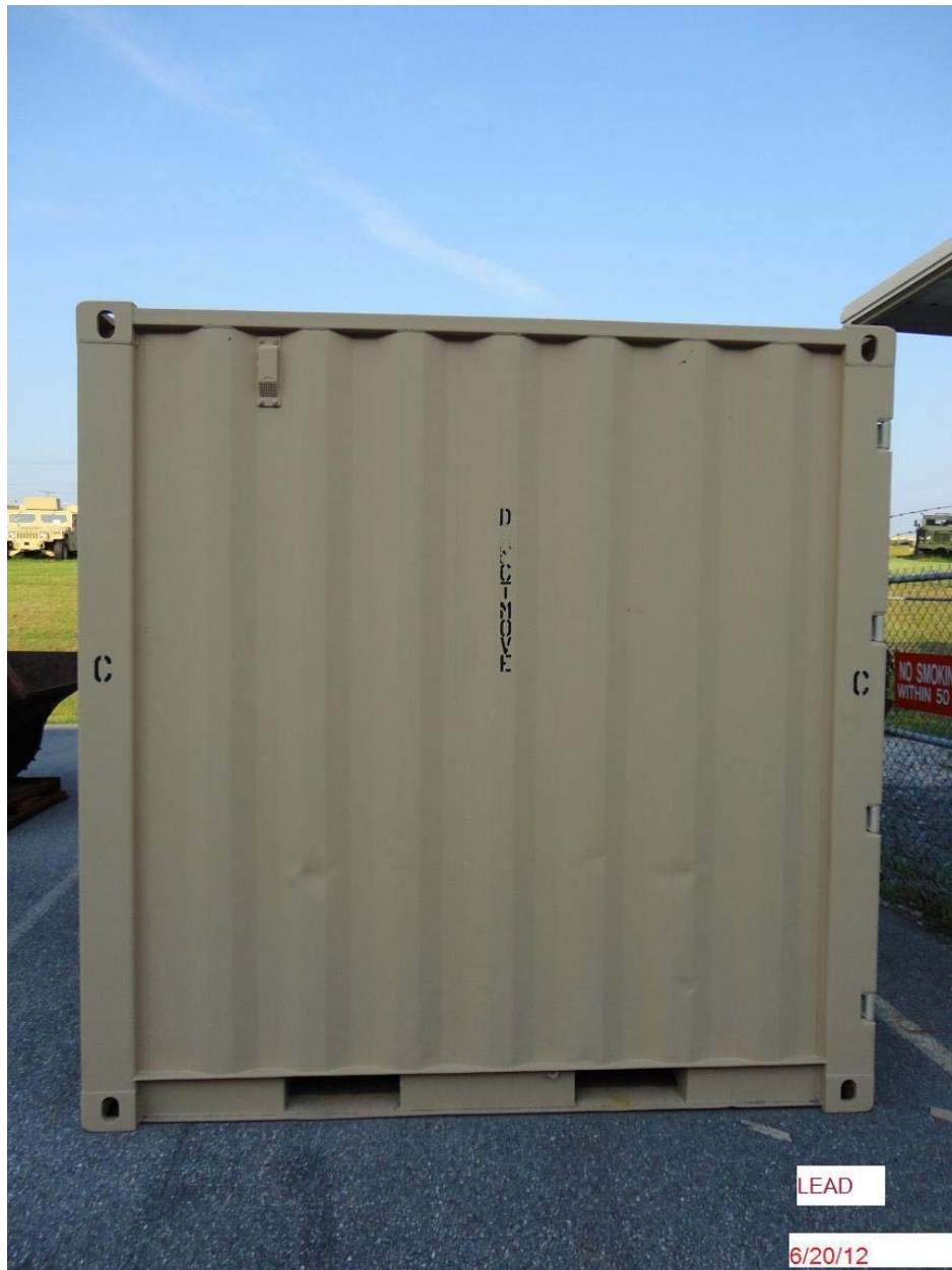
Figure 8. Tricon coated with Spectrum's experimental wash primer, MIL-DTL-53022 type III primer and MIL-DTL-64159 type II topcoat in tan 686a.
