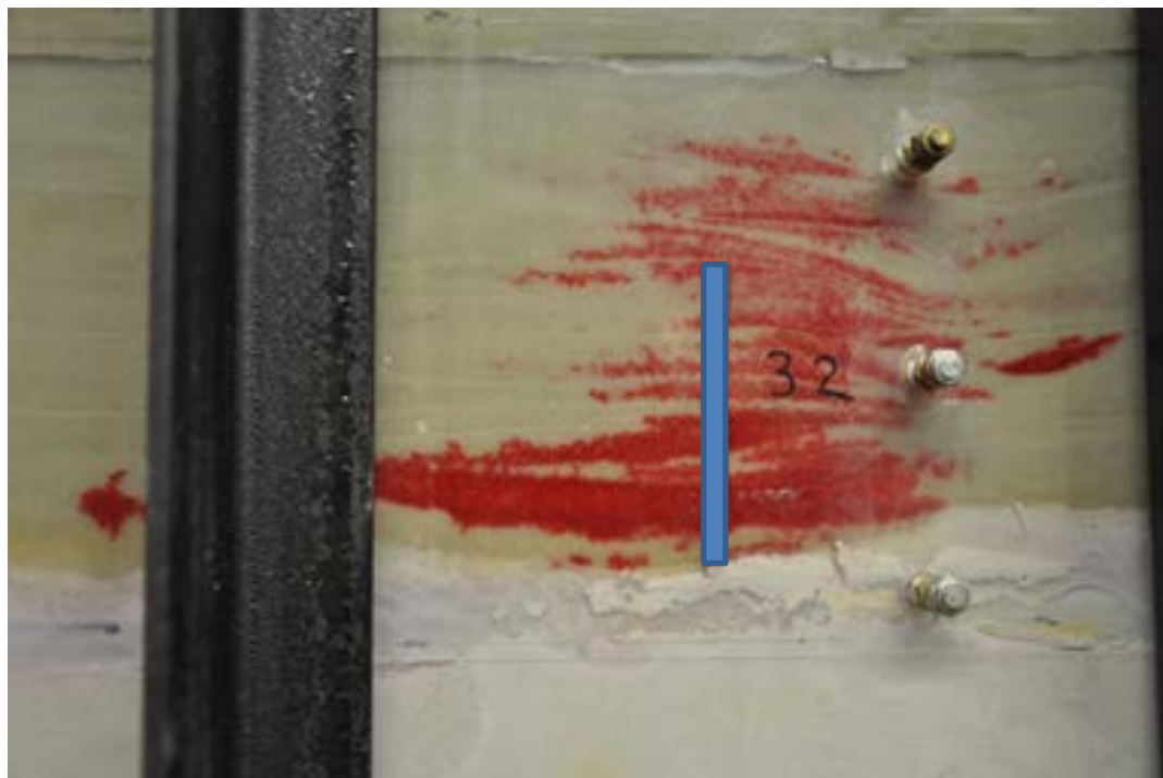
Figure 4. 6. Photograph showing the PCE DNAPL source zone created in the heterogeneous tank and used for the dissolution experiment. The blue rectangle represents the approximate location of the perforated portion of the injection tube.
