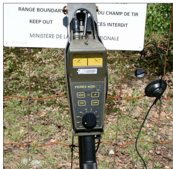
Figure 5-8. Forester metal detector used for proofing.
