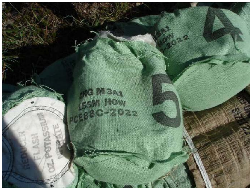
Figure 8-4. Gun propellant bags: M3A1, 155-mm caliber.
