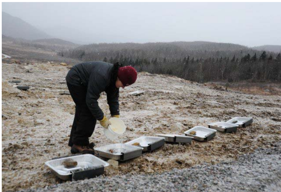
Figure 4-14. Particle traps in holders with weights.
