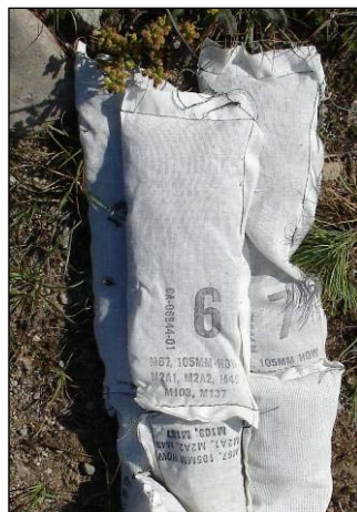
Figure 8-3. Propellant bags (M67, 105-mm caliber).
