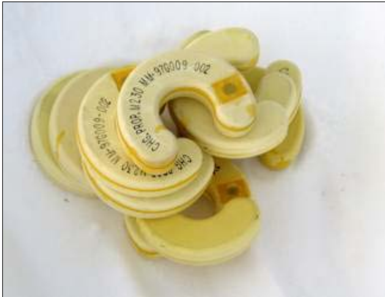
Figure 7-6. 120-mm propellant burn tests, charges on snow.
