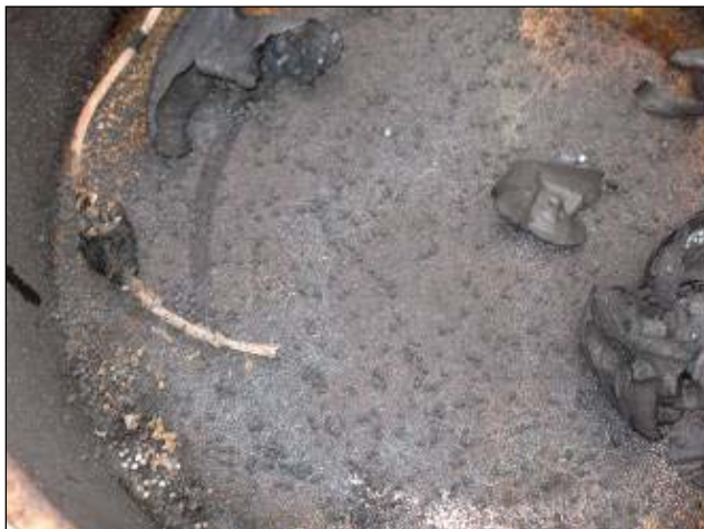
Figure 7-8. Aftermath of 120-mm propellant burn, residues in burn bowl.
