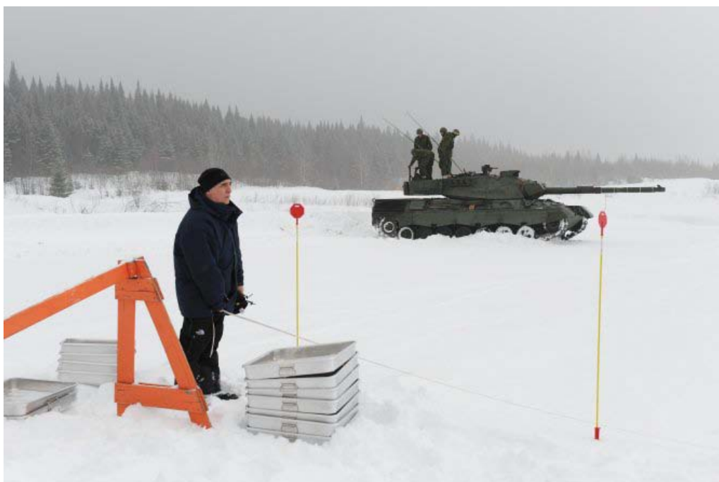
Figure 4-15. Stronger particle traps being installed on fresh snow cover.
