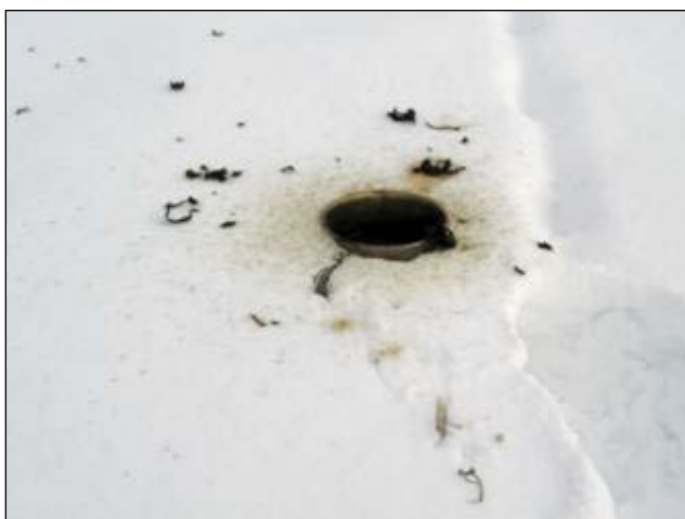
Figure 7-9. Aftermath of 120-mm propellant burn, residues surrounding bowl after burn.
