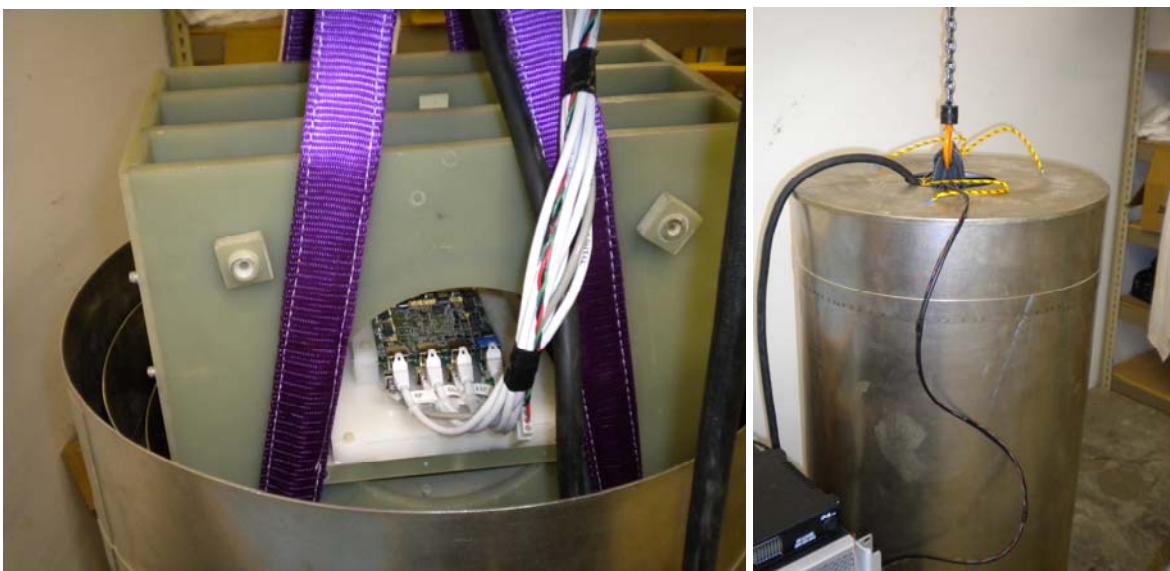
Figure 5. Photograph of the sensor board placed in the Helmholtz coil (left) and being lowered into a triple layered magnetic shield. Photograph of the sensor and Helmholtz coil installed inside the magnetic shield (right).
