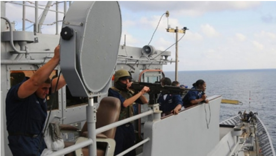
Figure 7. An example of LRAD operated onboard a naval vessel (From American Technology Corporation, 2004)
