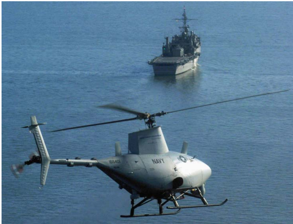
Figure 11. A Fire Scout prepares for the first autonomous landing aboard the USS Nashville (LPD 13) during sea trials in 2006 (From U.S. Navy, 2006).
