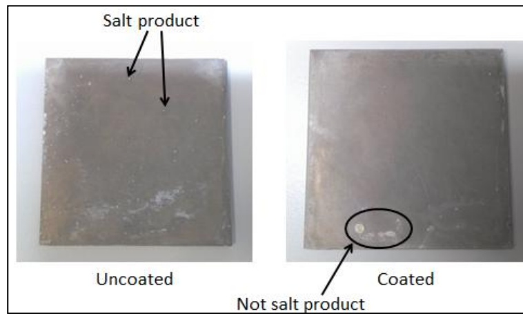
Figure 3. Comparison of uncoated and coated specimens after 14 days in salt fog chamber
