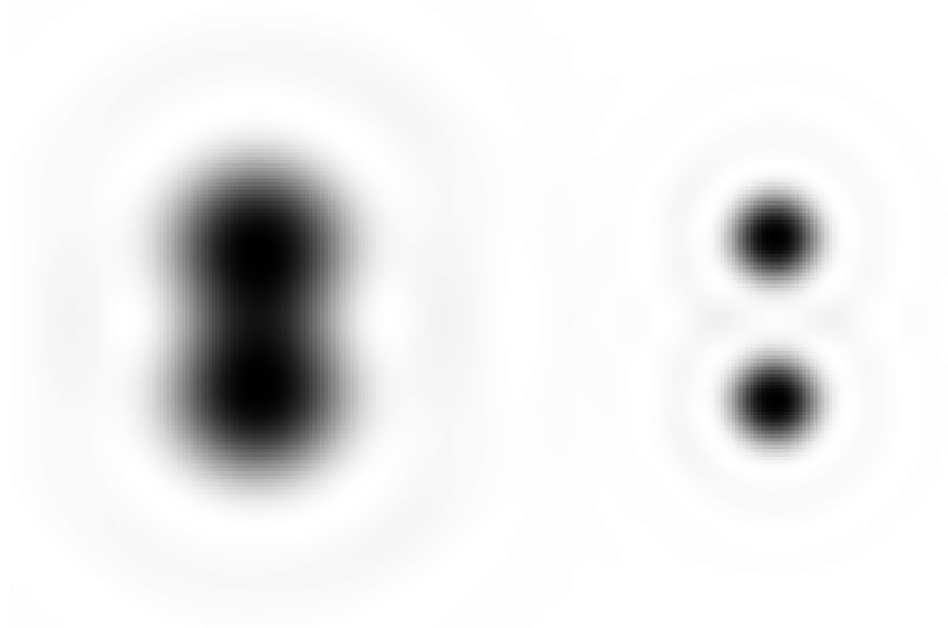
Figure 1.1 Simulated Airy's disks for two different aperture diameters. The aperture used for the images on the right side is double the diameter of the aperture used to form the images on the left side.
