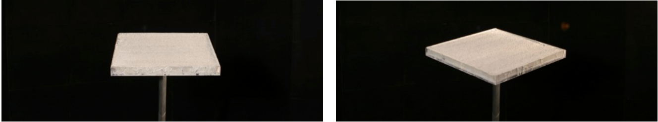
Figure 1: Photos of the brushed concrete on a low RCS pylon and tipped to 15 degrees elevation. The concrete is at 0 degrees azimuth on the left and 45 degrees azimuth on the right.
