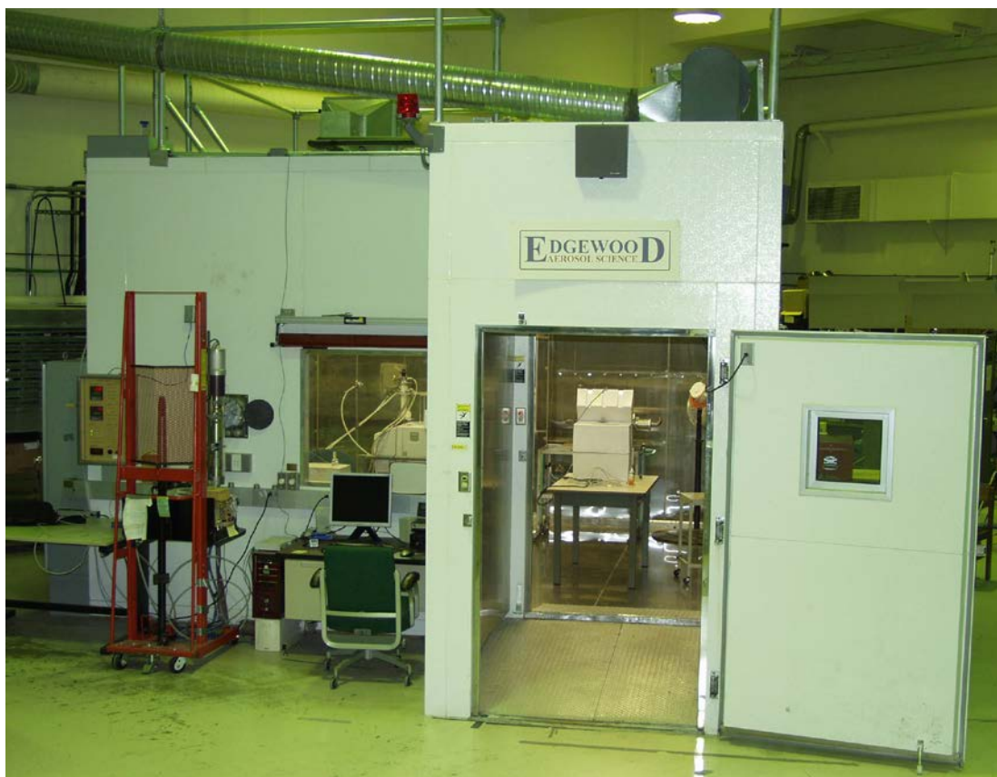
Figure 1 – Aerosol Deposition Chamber in Building E5951
