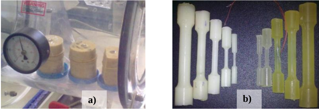
Figure 2. Hysol specimens in molds curing in a vacuum chamber a) and specimens obtained b).
