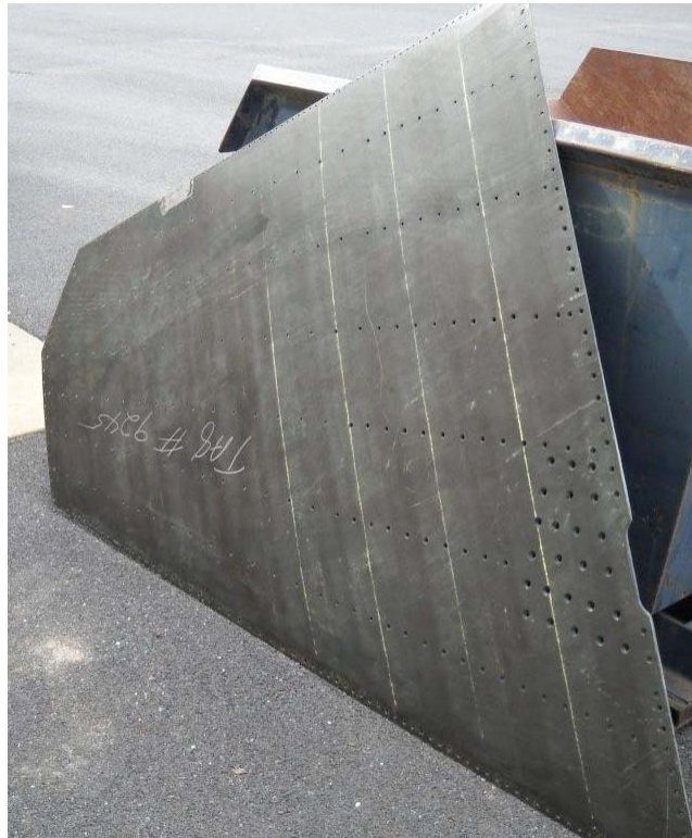
Figure 6.3. A picture of the scrap F-16 composite part before being cut. Five of the cut pieces were sent to FBS as test samples for demonstrating UMAT applications on realistic composite aircraft structures.
