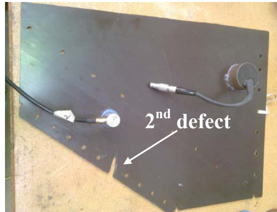
Figure 8.49. Picture of the 2 nd defect. The second defect was closer to the receiver than the first defect.
