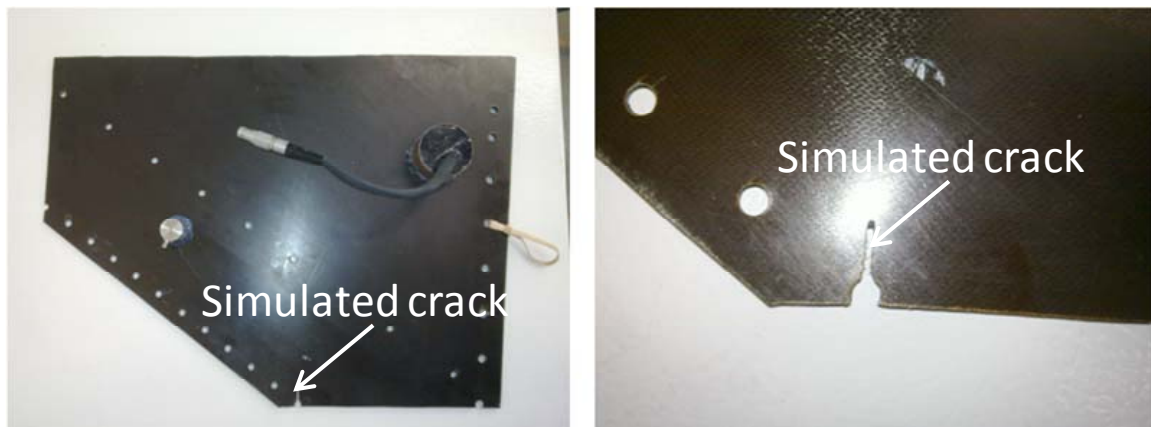
Figure 8.45. A simulated crack defect introduced to an open hole located at the edge of the test panel. (Left) Complete view of the test panel showing the simulated crack location. (Right) A close view of the simulated crack. The length of the crack was 0.5".
