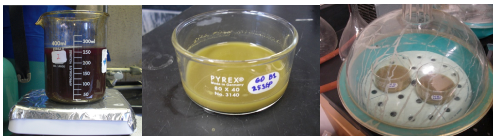
Figure 6. Left) Mixture of Graphite Powder with Acids and \text{KMnO}_4 and \text{H}_2\text{O}_2 at the end of the Reaction Time Middle) GO prior to being placed under vacuum Right) Nalgene Vacuum Desiccator with Graphite Oxide Drying.
