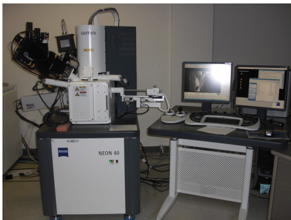
Figure 21. An image of the Zeiss SEM used to capture surface images of the samples.
