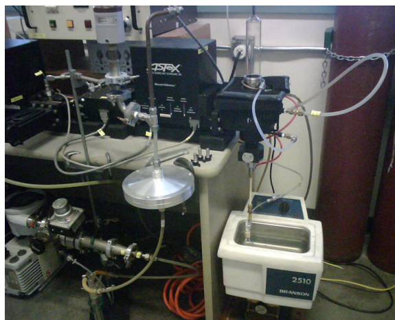
Figure 10. Aslex Atmospheric Microwave Plasma System used to create WO 3 .
