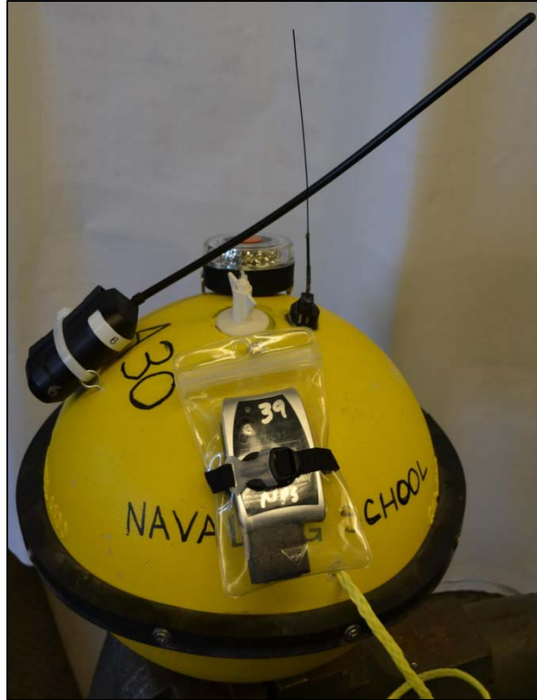
Figure 12. WRD Buoy. GT-31 GPS receiver (front), Garmin GPS tracking collar (left), Merlin RF transmitter (right) and NaviSafe marine light (back) are mounted externally on the buoy.
