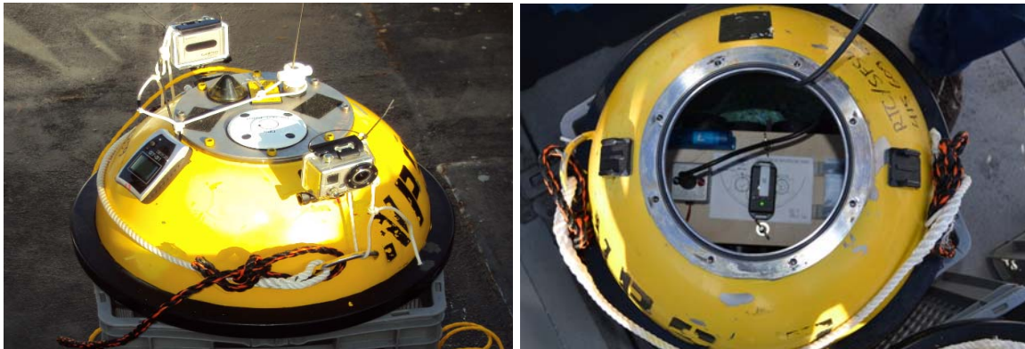
Figure 10. DWR-G external sensor configuration (left panel). GT-31 GPS receiver is visible on the bottom left. Two GoPro cameras are attached to the top of the buoy. DWR-G internal sensor configuration (right panel). The blue X6-2 accelerometer is visible in the top left of the internal board, while a Yost accelerometer (for future testing) is visible in the center.
