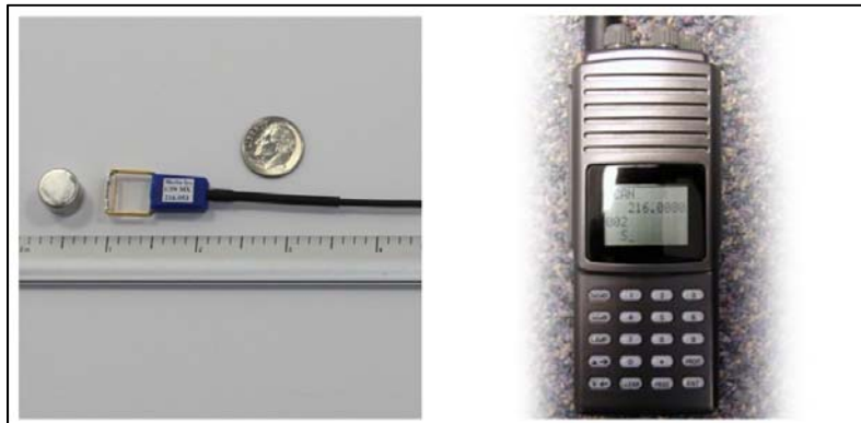
Figure 16. The left panel shows the Merlin 1/3N MX radio transmitter. The right panel shows the MS-1000 Multi-Channel receiver used for radio direction finding (From http://www.merlin-systems.com ).
