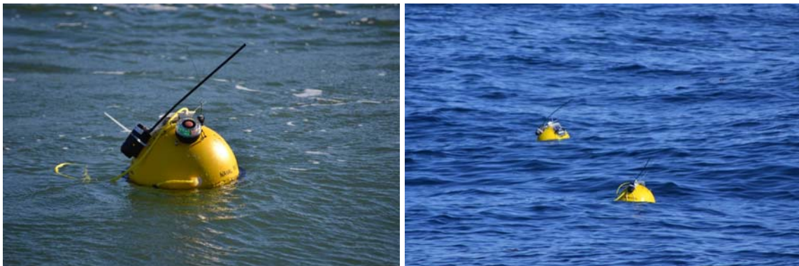
Figure 11. Wave Resolving Drifter (WRD) drifting inside Golden Gate Channel (left panel). WRD buoys drifting off of Monterey Bay, CA (right panel).
