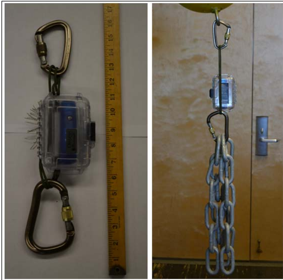
Figure 15. Tethered configuration of the X6-2 accelerometer. The X6-2 is secured inside a waterproof Otterbox and is ballasted by 20lbs. of chain link.
