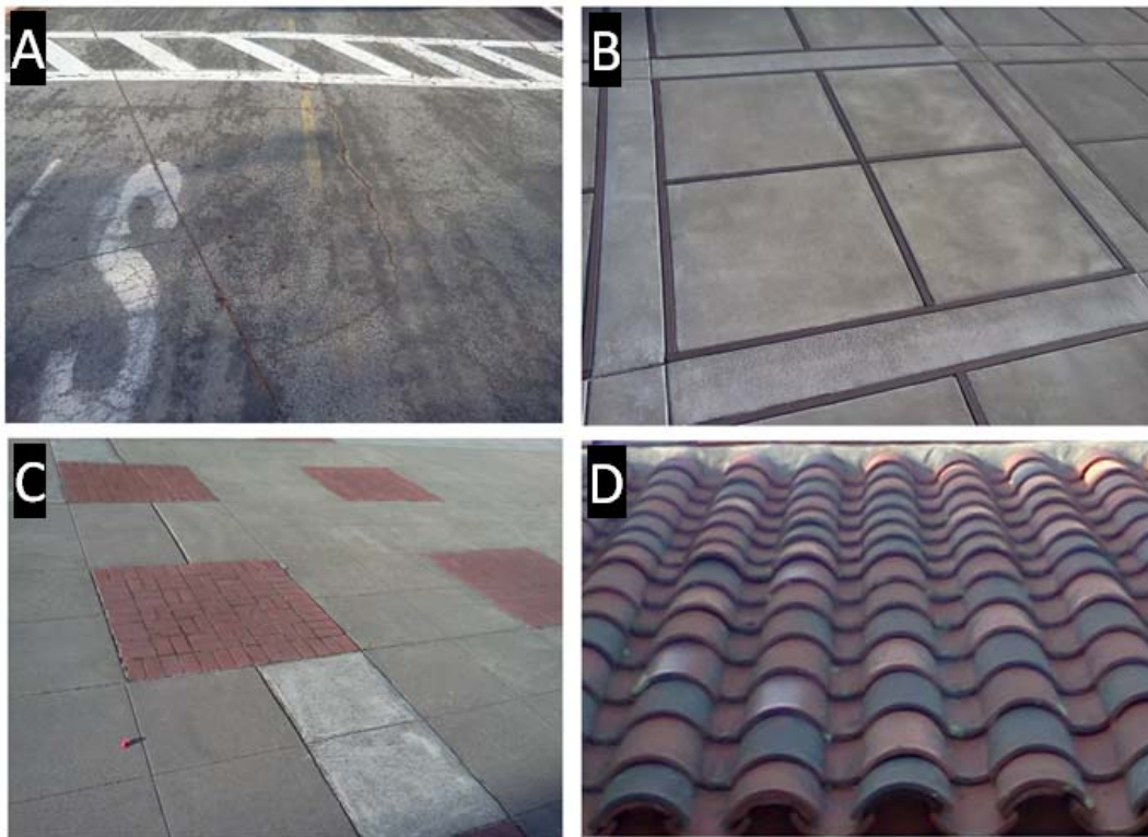
Figure 16. Various urban materials at NPS showing spectral variability within the FOV of a typical pistol grip foreoptic. Using the contact probe, each individual component is sampled. (A) Heavily worn asphalt with road paint (B) Two types of concrete with plastic border (C) Concrete with brick squares (D) Various clay roof tiles.
