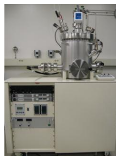
Fig. 1: Photograph of a growth system constructed for synthesis of graphene.
