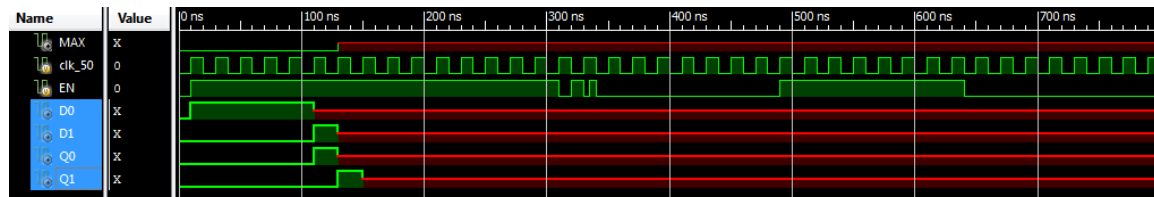
Figure 46. Timing diagram for the Moore-type FSM developed with output, clock, enable and D-FF input/output signals visible (floating-input case).
