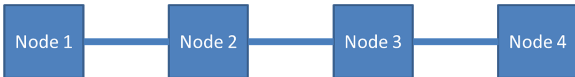
Figure 5. Linear Topology (Redrawn after [10])
